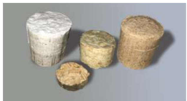
Brikett-Ø=40 mm Styropor / grobes Restholz / Weich- & Hartholz
