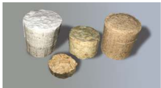
Brikett-Ø = 40 mm Styropor / grobes Restholz / Weich- & Hartholz
